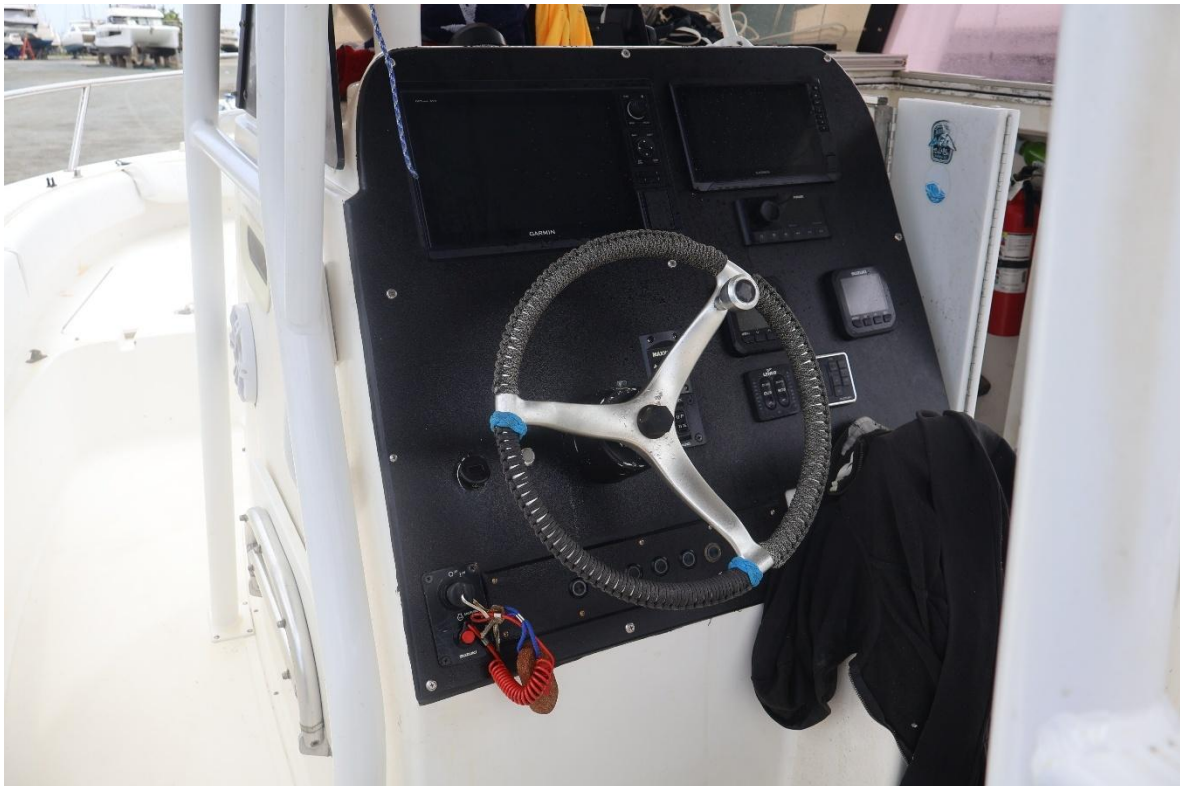
Figure 5: Kill cord connected to Kill switch and console.
