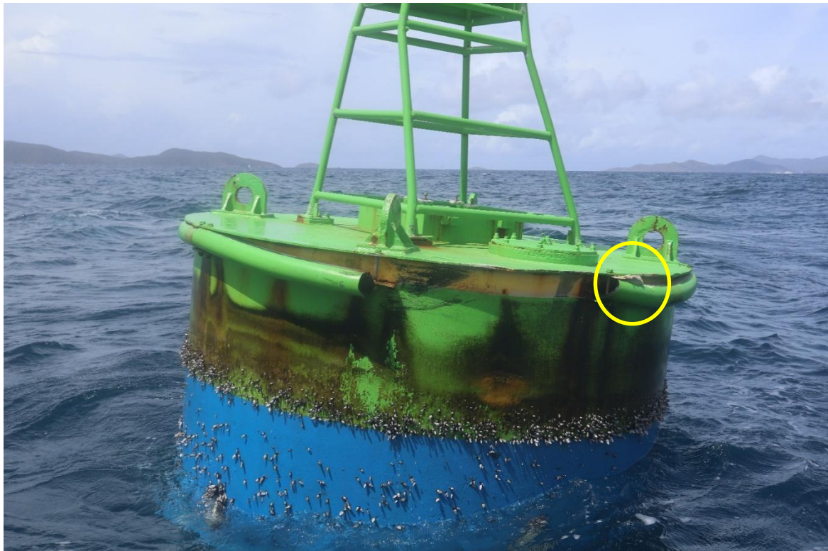
Figure 14: Pieces of fibreglass were observed stuck in the protective fender of the lateral channel marker's hull.
