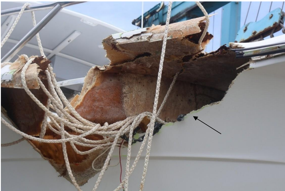
Figure 9: Green paint transfer observed along the damaged areas of the hull, consistent with the channel marker.
