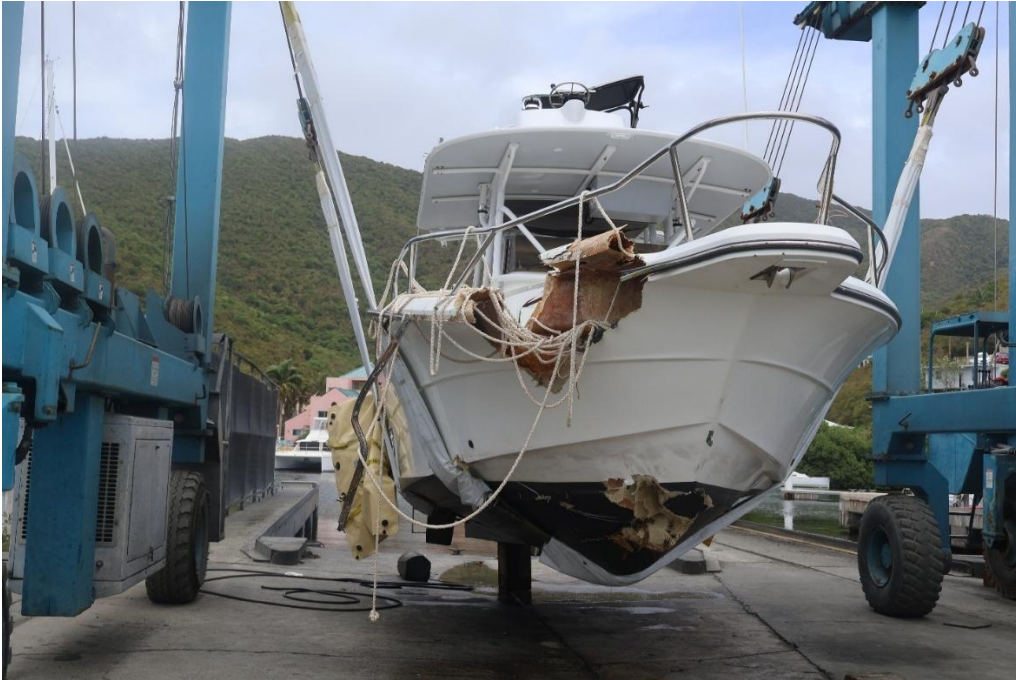
Figure 6: Severe damage to the bow as a result of the collision.
